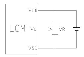
VDD~V0: LCD Driving voltage
